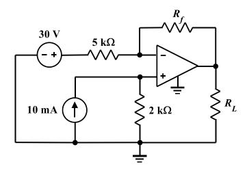
The OpAmp is ideal. Determine the value of  $R_f$  that will cause  $R_L$  to absorb NO power (0W).
